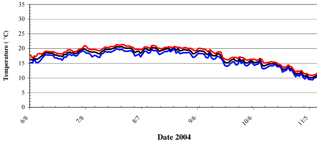
Figure 5-4. Daily mean (black), maximum (red) and minimum (blue) water temperatures at Station T-1 in Alameda Creek.
